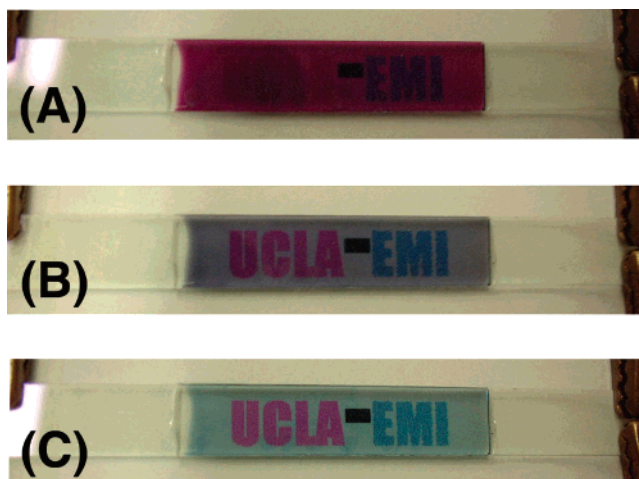
Figure 8. Colors of a sandwich-type P(BEDOT-MEHB) EC cell at three oxidation levels: (A) neutral, (B) intermediate, and (C) oxidized states.
